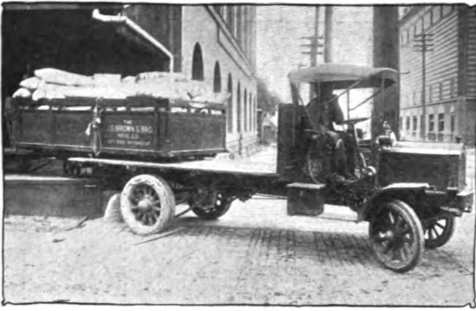
Special type truck body built for J. S. Brown & Brother Mercantile Company, Denver, Col., by the Packard Motor Car Company, Detroit, Mich. Detached bodies may be rolled on channel irons in the truck platform.
